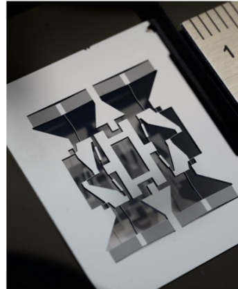
(a) One of the kinematic configurations of the novel rectilinear stage family. (b) Flexure-based implementation of the mechanism in deformed position. (c) Fabricated silicon rectilinear flexure stage preloaded by thermally oxidized buckled beams for stiffness reduction along the translational direction.
