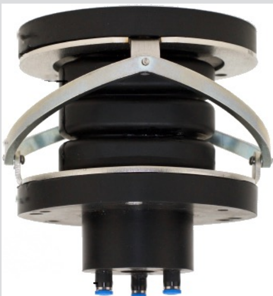
Hard-soft actuator with joints for precision movements and pneumatic chambers for adjusting the stiffness and effectuating bending motions
