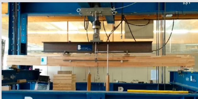
With the innovation of laminated beech wood, beams with a bending strength of over 60 megapascals (MPa) are possible.
