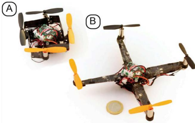
**Figure 1.** Miniature quadrotor equipped with foldable and self-deployable arms. (A) Stowed configuration with the arms wrapped around a central rigid frame. (B) As soon as the propellers are activated, the arms autonomously deploy and the quadrotor unfolds to a ready to fly configuration. The control board, battery, motors and propellers belong to the commercial quadrotor Walkera QR Ladybird.
