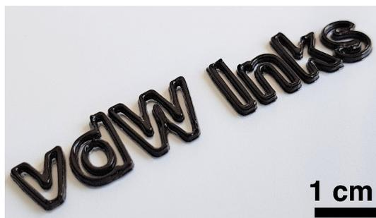
The inks are specifically suited for extrusion- and screen-printing. Further applications are in the field of stretchable wires and interconnects, embedded electronics, self-healing circuits, conformal electrodes, heat transfer systems, and thermal cooling and heating designs.
