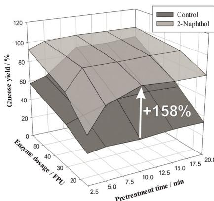
Fig. 1: Enhancement of glucose yields in enzymatic hydrolysis. Steam explosion pretreatment: 1.5 kg spruce wood, 35 g 2-naphthol (scavenger) or no additive (control),  $T=235^{\circ}\text{C}$ ; Hydrolysis: 1% w/w cellulose, 15/30/60 FPU/g cellulose
