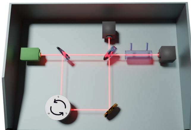
fig. 2 Modified delay-line with continuously rotating mirror assembly, which increases the data acquisition rate.
