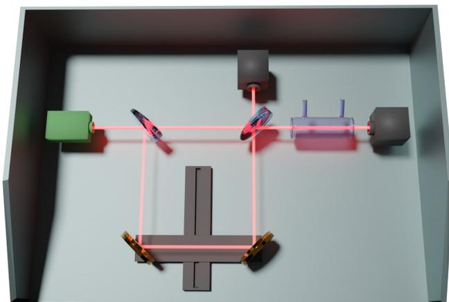
fig. 1 Conventional set-up of an FT-IR spectrometer with linearly displacing mirrors.
