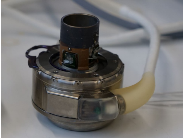
(left) The Abbott HeartMate 3 with modified inflow cannula, (right) scheme of cannula with two embedded pressure sensors.
