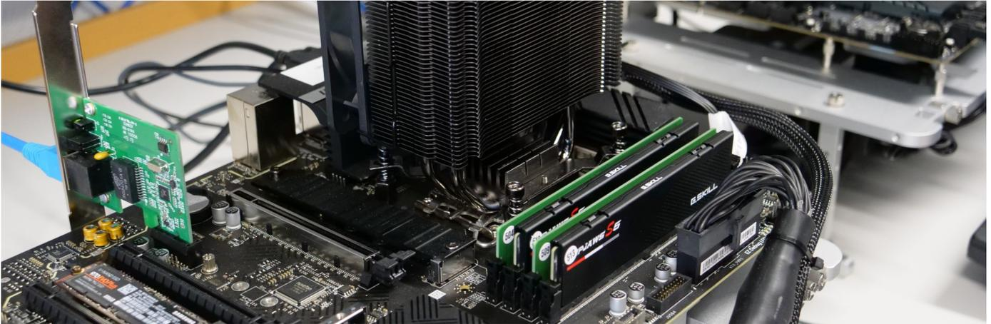
Photo: Test-rig for DRAM modules. Over 40 modules of various manufactures showed vulnerability to sophisticated Rowhammer attacks. The presented method protects against Rowhammer and is easily integrated into the hardware.
