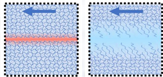
Oxygen supply during polymerization influences the lubricity of the surface layer. (left) Low oxygen supply causes high cross-linking and high friction. (right) High oxygen supply inhibits cross-linking and lowers friction.
