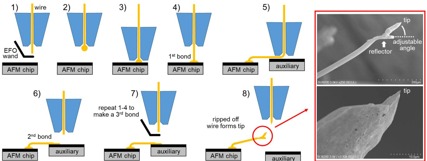
An Electronic Flame Off (EFO) wand melts the wire forming a ball, which is then pressed against the AFM chip, forming a strong first bond. The second bond is established by only pressing down the wire on the auxiliary chip. Steps 1-4 are repeated to form a third strong bond at the end of the cantilever. The wire is ripped off quickly to form the fine AFM tip.
