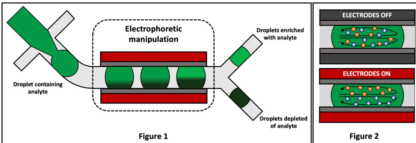
Fig. 1) Schematic concept of a microfluidic device, comprising a droplet generator, a flow channel for electrophoretic enrichment and a Y-junction for droplet splitting. Fig. 2) Migration of charged molecules within the moving droplet without and with an applied electric field.
