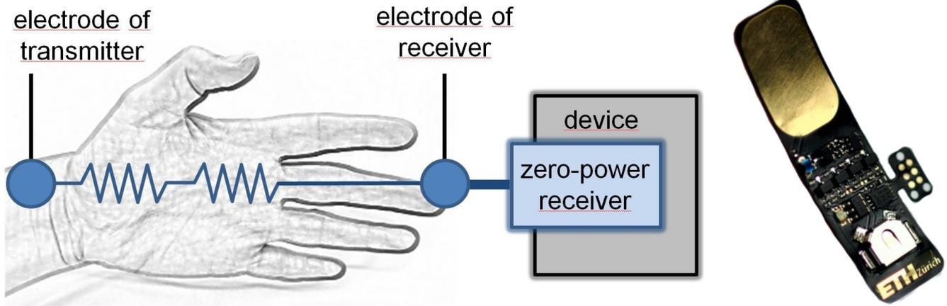
Fig 1. (left) Upon touch the transmitted signal first charges the receiver and then passes its data. (right) Prototype of the zero-power receiver
