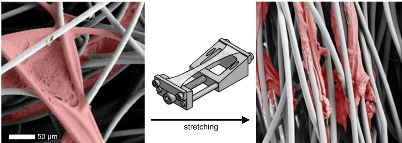
Fig 1. (left) False colour electron microscope image of unstretched scaffold visualizing the connection between the PGA and P4HB polymers, (middle) stretching the elastic scaffold, (right) stretched scaffold with aligned fibres [1]
